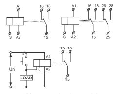
It is possible to connect load between S-A2 (e.g contactor, control of light or any other device, without disturbing a correctgunction of relay(load is energized while the switch is ON.)
